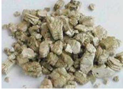
Zonolite Attic Insulation ("ZAI")
